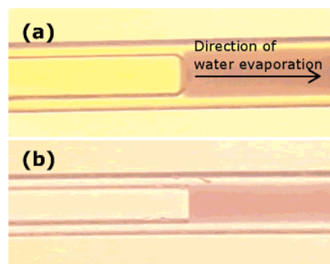
Figure 2. (a) Optical microscope image of colloidal assemblies inside a 50 \mu\text{m} diameter silica microcapillary. (b) Optical microscope image of colloidal assemblies inside a 65 \mu\text{m} diameter polymeric microcapillary.
