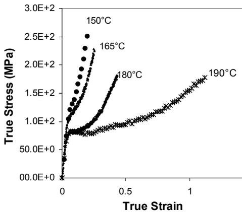
**Fig. 1 Room temperature stress-strain characteristics of 200 micron diameter PMMA fibre drawn at various temperatures.**
